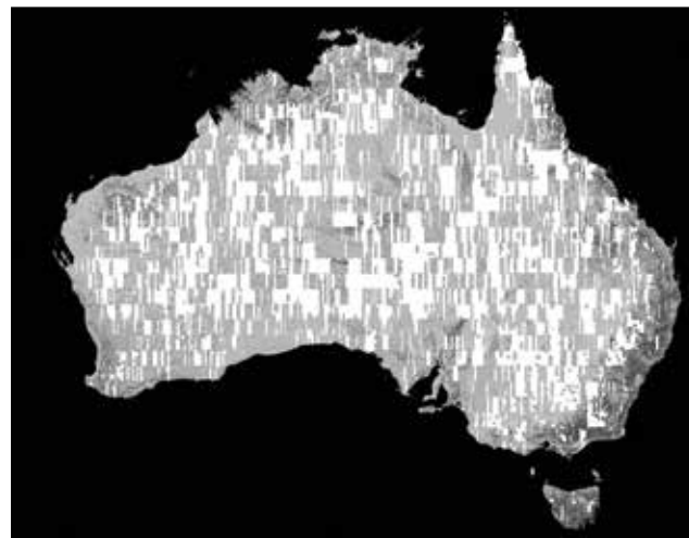
Figure 1: Map of the topography of the current production status of Australia. Each strip of elevation data is acquired in a single pass by Worldview-1, -2, or -3 and is processed on Blue Waters.
