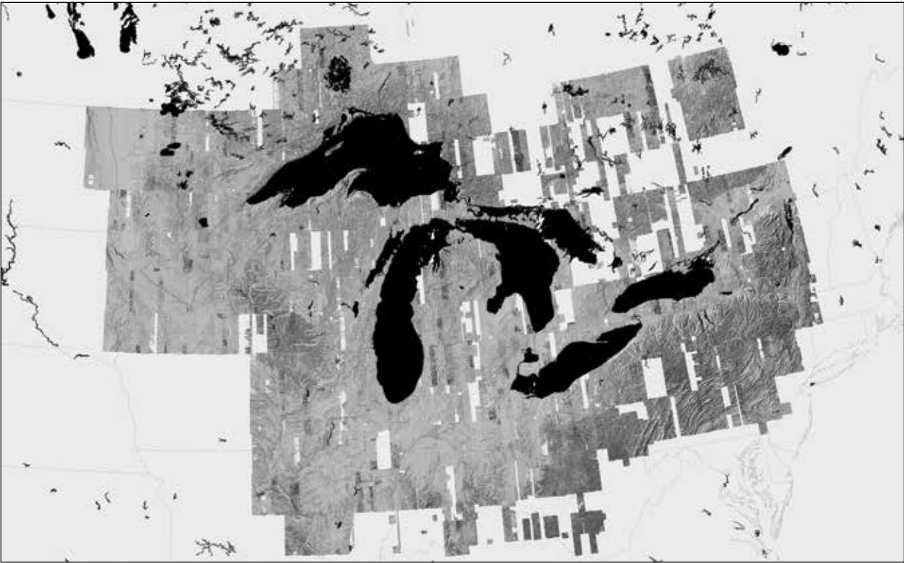
Figure 1: Great Lakes Basin digital surface model (DSM) production status as of May 2019. The source of the stereo imagery used to produce these DSMs spans the archive, starting in about 2008 to early 2019 (2019 DigitalGlobe NextView License).
