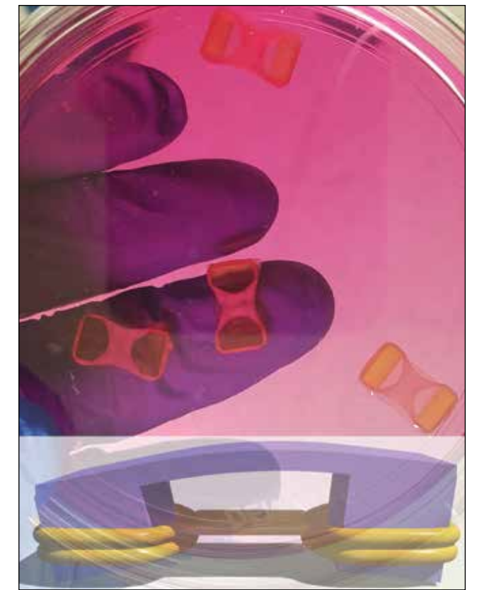
Figure 2: Top view of three thumb-sized biobots in a culture dish. Modeling and simulations were employed to design and optimize function and performance. These biohybrid machines walk on the dish surface at about one millimeter per second.
