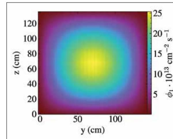
Figure 1: This image shows the neutron flux in a 2D cylindrical axisymmetric model of a molten-salt reactor. This flux has the anticipated magnitude and canonical cosine shape ( $r = 0$  is center of core) and is undergoing validation against experimental results from the Molten-Salt Reactor Experiment.
