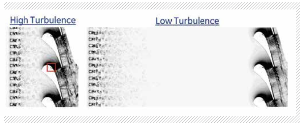
FIGURE 2: Numerical schlieren for a cooled transonic vane at 5% and 20% turbulence intensity for unstructured second order solver.
