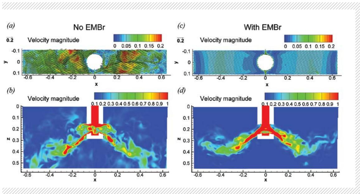
**FIGURE 4:** Predicted velocity in a horizontal plane near the top surface (top) and in the middle vertical plane of the caster mold (bottom) for cases without (left) and with (right) an external magnetic field.
