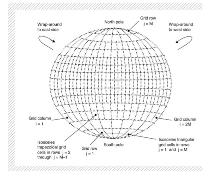
**FIGURE 1:** Layout of the 3D FDTD grid as seen from a constant radial coordinate.
