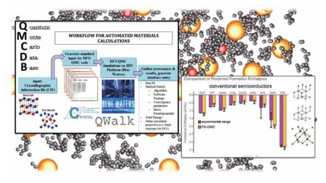
Figure 1: Background: a snapshot of a configuration of electrons around atomic nuclei in the magnesium oxide solid. Foreground: the Autogen workflow for automated quantum Monte Carlo calculations of solids and incorporation into quantum Monte Carlo database, and selected results for calculated formation enthalpies of conventional semiconducting solid materials.
