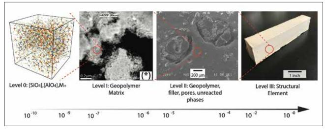
Figure 1: Multiscale nature of geopolymer composites. Our study spans levels 0 at the nanometer length-scale to level III at the macroscopic level.
