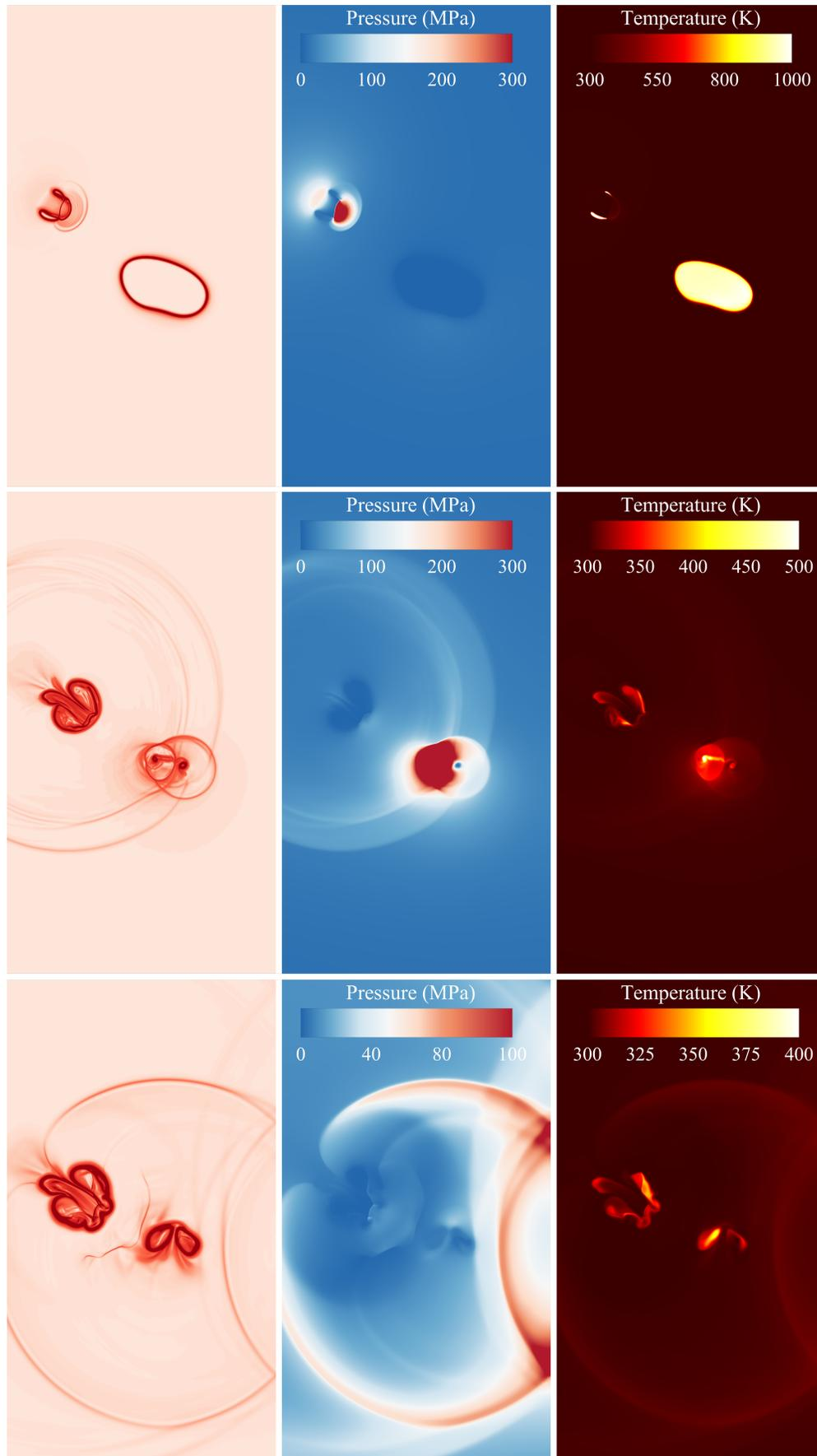
Figure 4: Collapse of a bubble pair near a solid wall. 2D slices of numerical schlieren (left), pressure (middle), and temperature (right) fields during the collapse.
