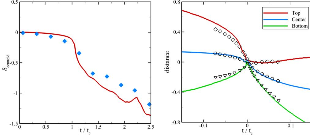
Figure 2: Left: bubble centroid as a function of time; right: time history of the bubble walls and the centroid location around the time of the jet impact. Solid lines: numerical solution; symbols: experiments.
