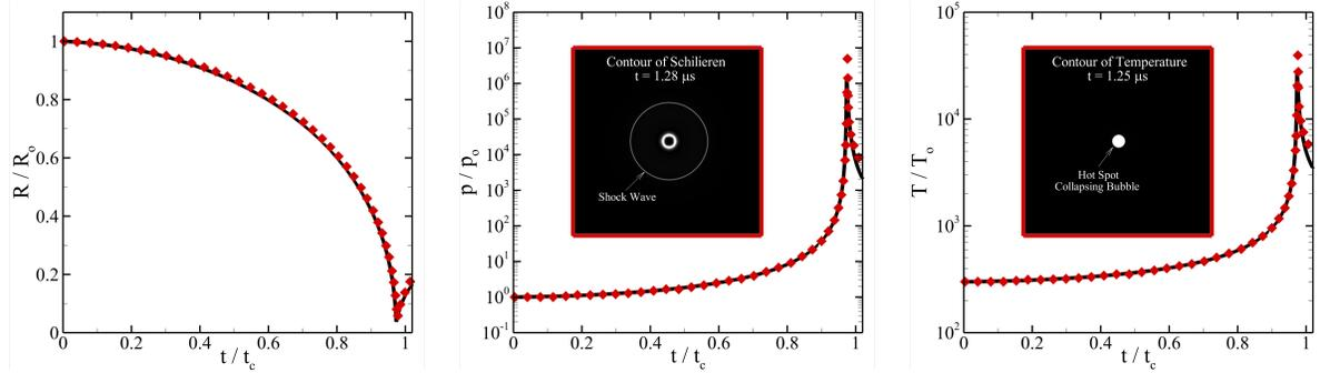
Figure 1: Spherical collapse of an isolated vapor bubble in water. Black solid line: KM solution; red diamonds: numerical simulation.
