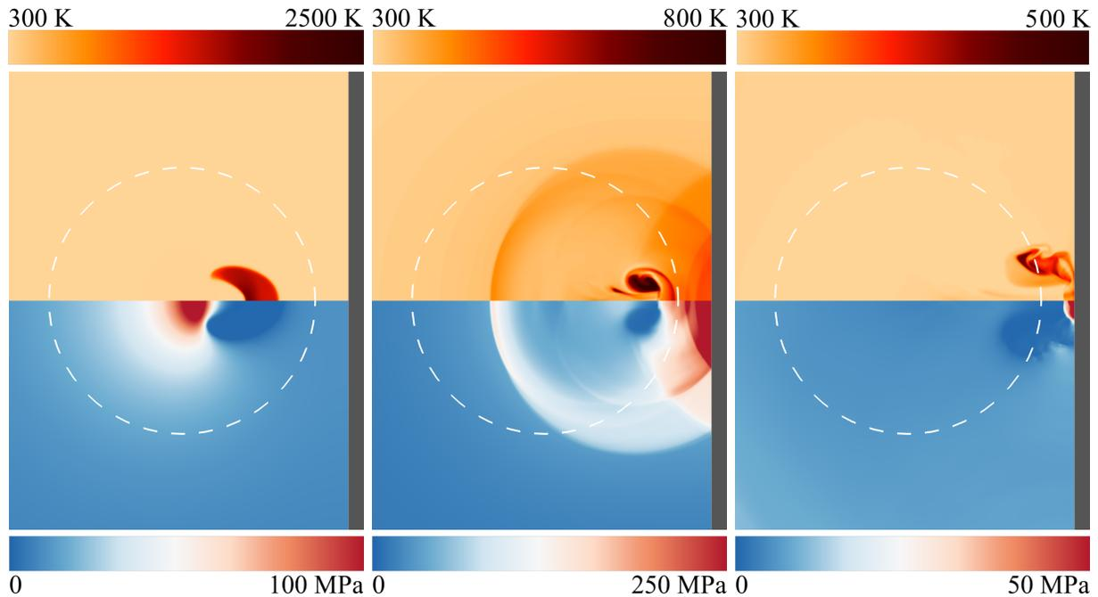
Figure 3: Collapse of a single bubble near a solid wall. 2D slices of temperature (top) and pressure (bottom) fields during the collapse; white dashed line: initial configuration of the bubble.
