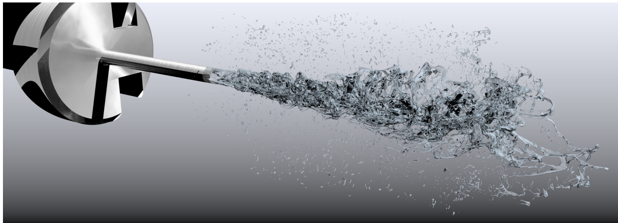
Figure 1: DNS of a scaled-up injector at high-density ratio (800), low Reynolds number (5000) and moderate Weber number (60000) conditions.
