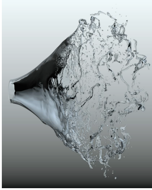
Figure 3: A pressure-swirl atomizer.
